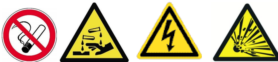
Figure 2-10: Warning stickers to be installed close to the battery bank in the technical room
