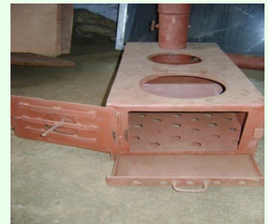
Figure 6 Model -IV ( 2 pot hole with ash tray)
