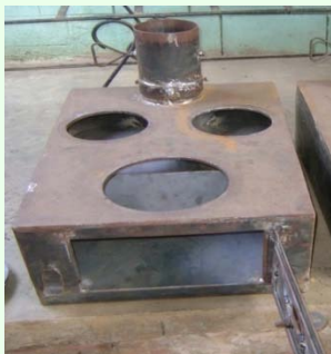
Figure 2 Model -II (3 pot hole metallic stove)
