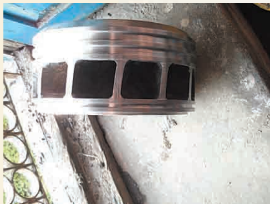
Runner of a 33 kW Micro Francis Turbine.
