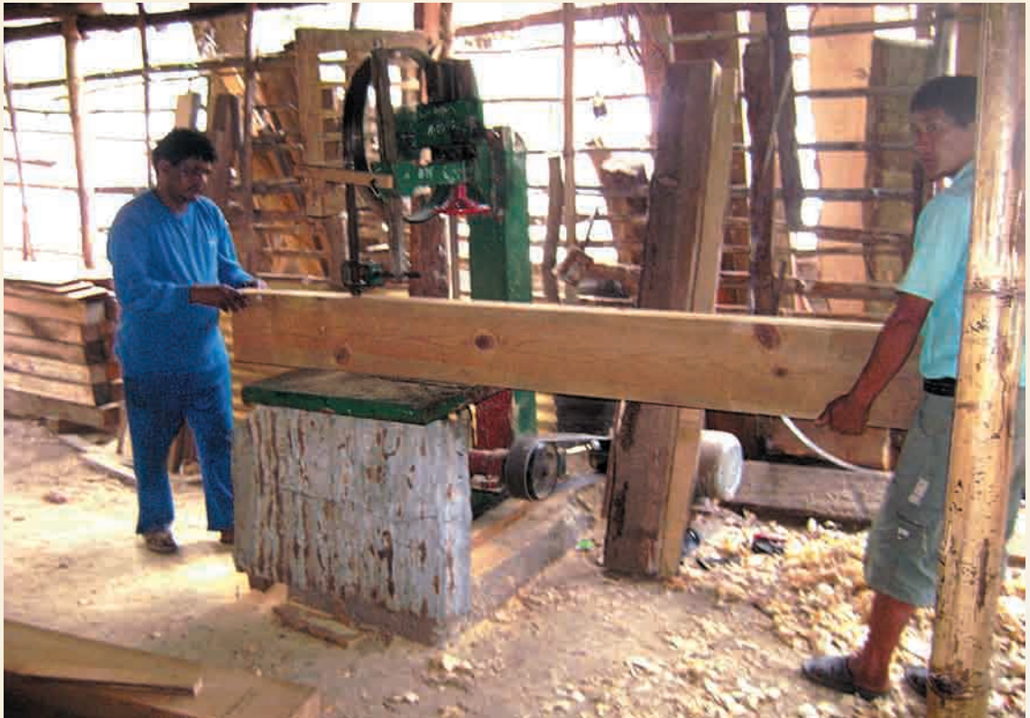
Saw Mill driven by a 22kW Micro Hydropower Plant in Burtibang of Baglung supported by the ESAP.
