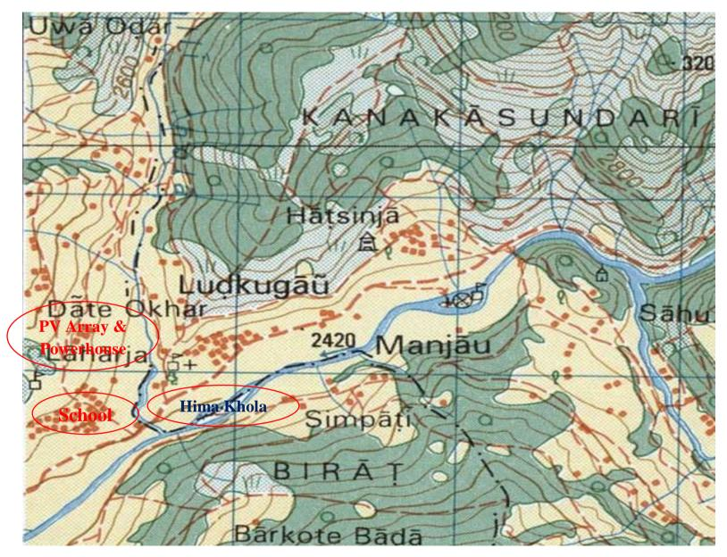
Figure 2: Topographic Map of Kankasundari Solar Mini Grid Subproject
